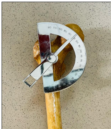
Fig. 3. Measurement of neck-shaft angle of Femur using Goniometer
